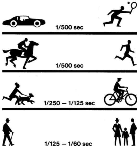
In general: Movement at close range and across the viewing direction needs faster shutter speeds, movement from greater distances and approaching or receding from the camera allows slower shutter speeds.
