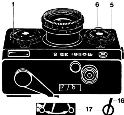
With the camera held in this way: Turn the aperture dial 5 to bring the red matching pointer 17 into line with the meter needle 16. If necessary select a longer or shorter exposure time.
