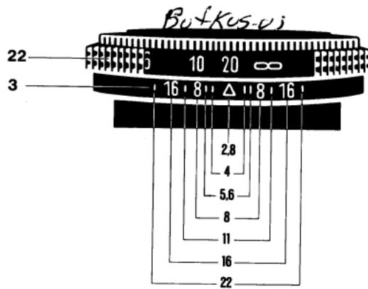
For distant views with near foregrounds set the infinity marking  $\infty$  opposite the aperture in use on scale **3**. That extends the depth of field to the nearest possible point in the foreground.
